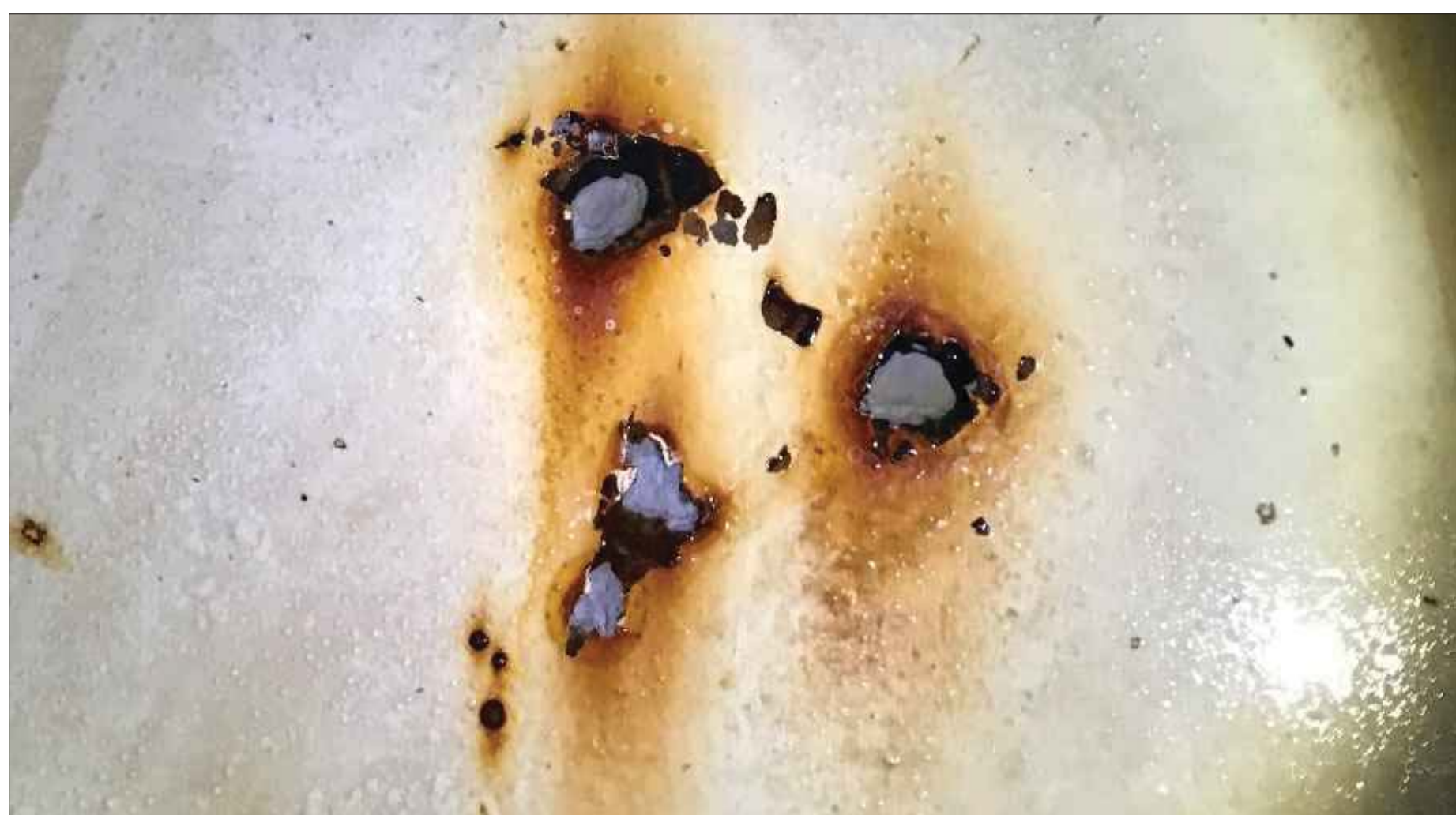
Figure 16. Tank Bowl Interior Repair pitted tank bowl as viewed from interior of the tank
