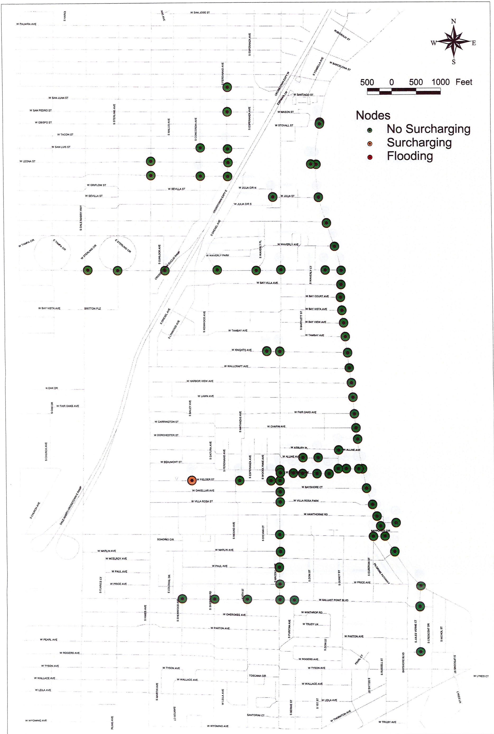
Figure 4-3. Alternatives 1, 1A, & 1B - Upgrade Bayshore Pump Station to 6000, 8000, & 10000 gpm Coachman Avenue Overflow Elimination Study
